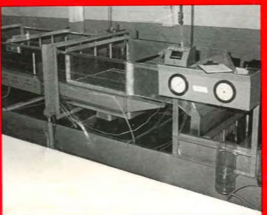
Laboratory and full size flume used to test grates for data appearing in this report.
